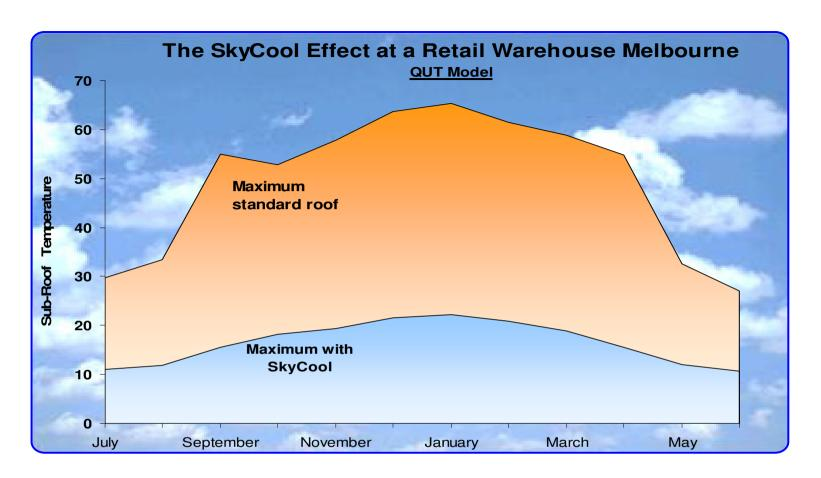
A large retail centre in Melbourne was experiencing difficulties with over heating during the warmer months. It was recognised by the centre's consultant engineers that the majority of the heat was entering through the roof from the solar load. A normal galvanised metal roof will often attain temperatures approximately twice that of the ambient shade temperature – on a 30 °C day, the roof can be as much as 60 °C transforming it into a large overhead radiator.
